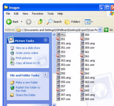
Figure 11-8. Images Folder has Four Formats per Data File: JPEG, Angle, Calibration, and Orientation
